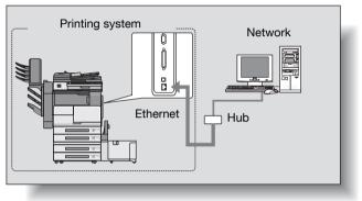
This printing system supports 10Base-T and 100Base-TX standards. In addition, the Ethernet interface supports the TCP/IP (LPD/LPR, Raw, IPP, SMB), NetBEUI (SMB), IPX/SPX (NetWare), AppleTalk (EtherTalk) and Bonjour/Rendezvous protocols.
